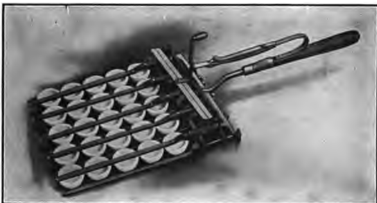
FIG. 28.—MULTIPLE SCORIFIER TONGS. (Keller.)
